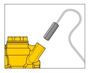
This system allows disinfection control in each circuit and optimization of the disinfection process. In this case it is possible to measure and monitor the water temperature in each circuit, even from remote.
