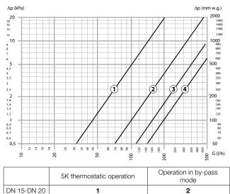
To choose the recirculation pump head, the head loss at the valve should be added to the head loss in the most disadvantaged circuit.
