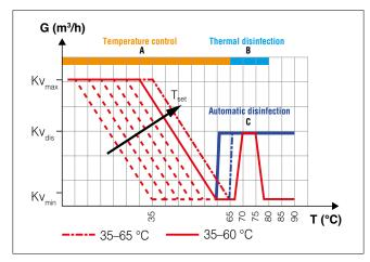
The graph shows the variation of the Kv value depending on the device configuration (A, B, C) and on the inlet temperature of the domestic hot water.
